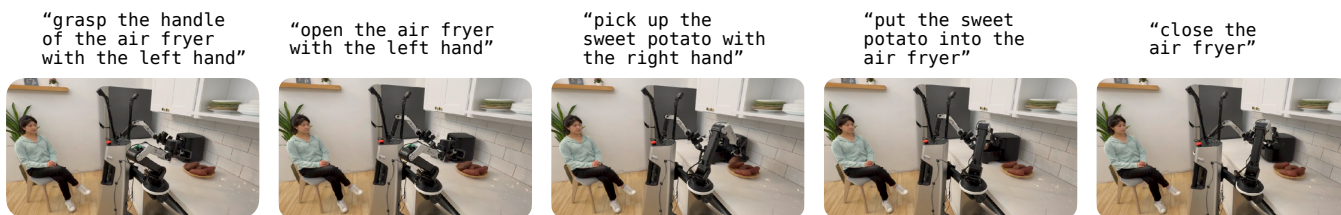
Fig. 14: Example of language coaching: We can “teach” a new task to \pi_{0.7} by providing step-by-step verbal instructions. Because of its language following ability, \pi_{0.7} can perform new tasks successfully under user instruction, and these instructions can then be used to train a high-level policy that prompts \pi_{0.7} so that it can perform the task fully autonomously.
